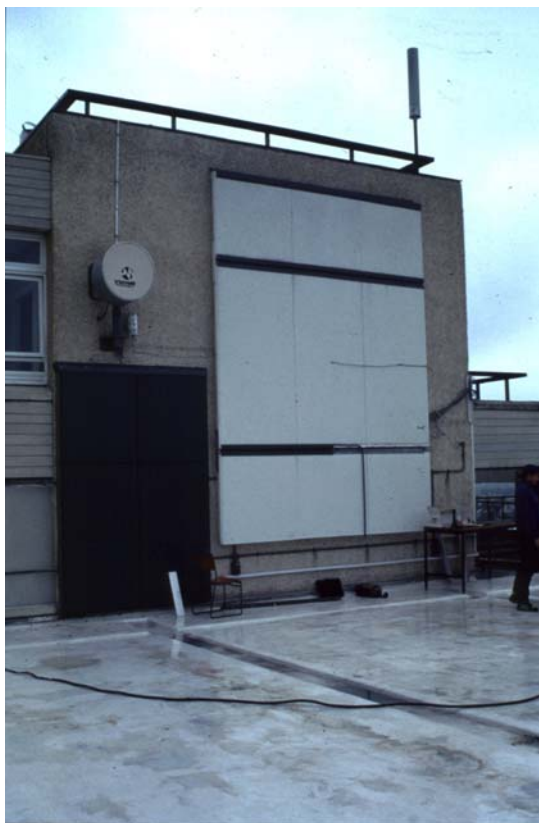
Figure 9 Edinburgh University over-cladding test
